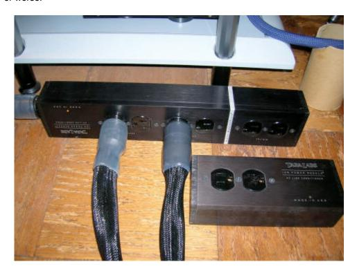
The TARA passive conditioners come in two models. The PM/2 Power Screen (\$395) is impressively machined out of thick, black, mil-spec aluminum, with an overbuilt, rather than luxurious, appearance (personally, I would like to see rounded corners and a smoother finish). It sports a detachable power cord, surge protection, one duplex outlet, an amber pilot light, and treatment for noise reduction, which we will get to shortly.
