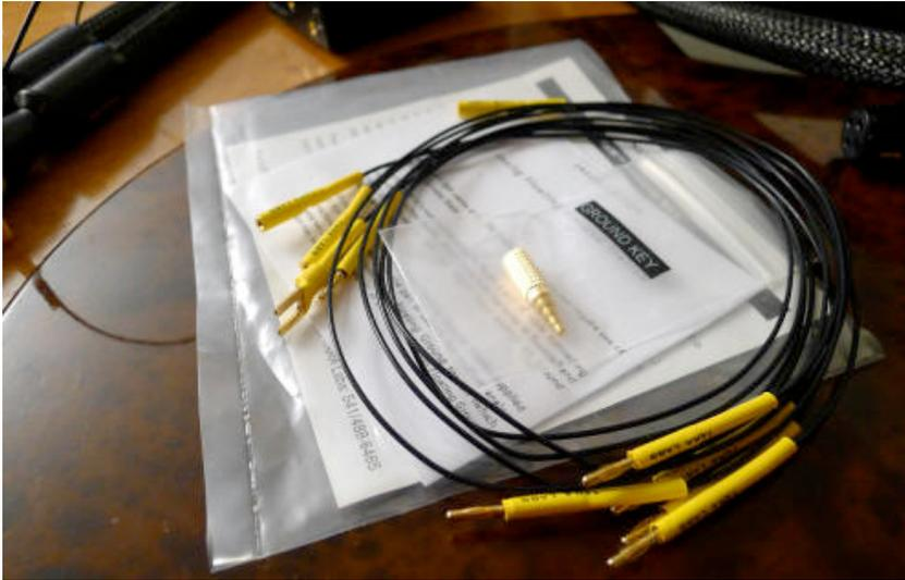
Like the upper-end TARA cables, the Air Evo interconnects have pigtails sprouting on both ends. The source side of the cable has mini-bananas that plug into the outboard EVO Floating Ground Station (FGS). The EVO FGS, in turn, is connected via mini-banana pins to ground somewhere on the component's chassis. In this way, the EVO FGS provides an independent ground path.
