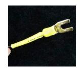
c) To use the Chassis Ground Key, locate a screw at the rear of the component chassis and remove the screw. The best location would be preferably the top rear corner, if possible. Then, the Chassis Ground Key is screwed in to the screwhole of the component chassis. The multiple threads at the tip of the Ground Key will ensure a tight mechanical connection to the component chassis ground. Or just loosen the screw, insert the mini spade and tighten.
