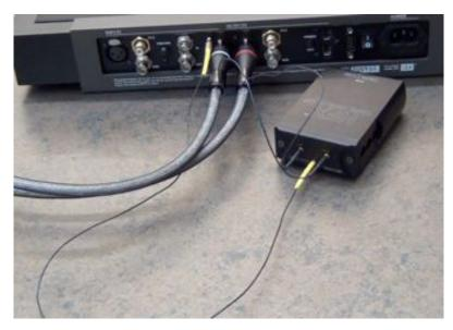
**TECHNOLOGY NOTE:** When combining the interconnects to the HFX Floating Ground Station, the Shield will be 'floated', not connected, to the circuit ground or (-) signal run of the cable. Instead, the HFX Floating Ground Station will provide an independent ground path and absorb RF/EMI energy in the shield, thereby lowering the noise floor for a much quieter cable as well as enhanced details.
